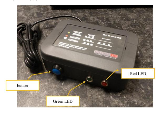
**Button**: used to put the module in pairing mode when pressing shorter than 1 second or clear the paired devices list if pressed longer than 3 seconds.
