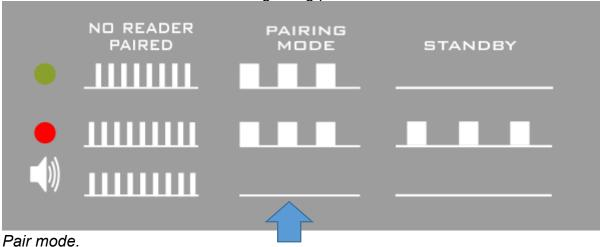
The base station will remain in pair mode for 10 seconds after the button has been pressed.
