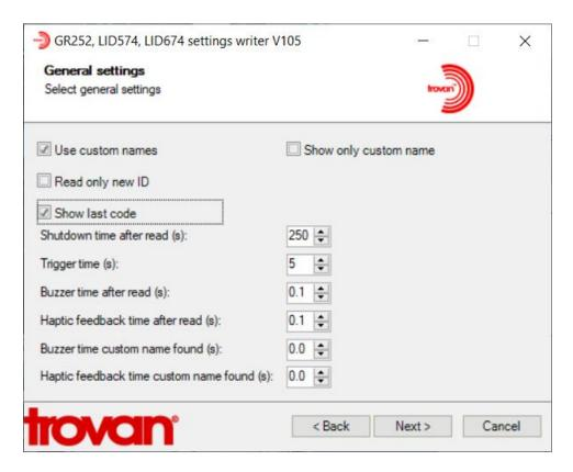
Or to reduce battery Consumption (reduce the shutdown time after read interval)
