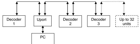
The LID665N decoders and the LID650N decoders can be used together in the same RS485 network.
