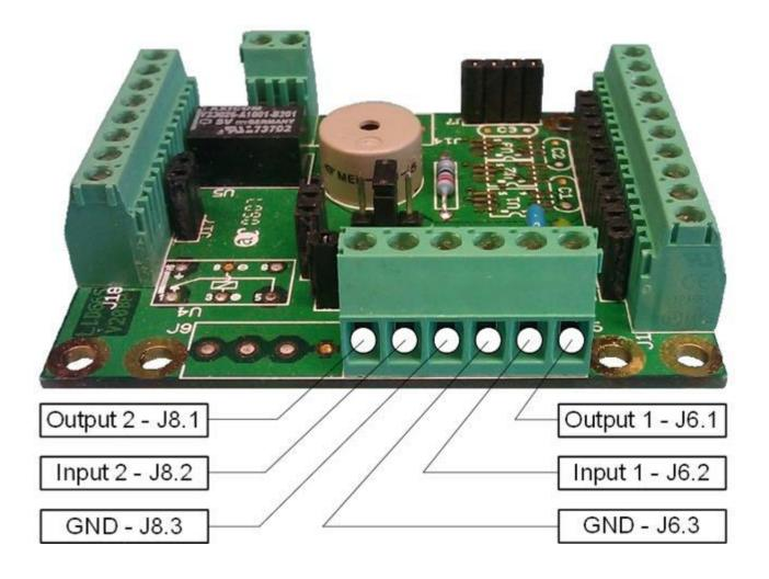
NOTE: Use pull-up or pull-down resistors for the sensors (depending on the sensor type) Never exceed VCC (5Volts) on the sensor input pins
