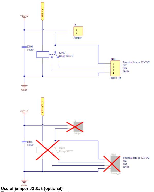
The two jumpers can be used in two different ways.
