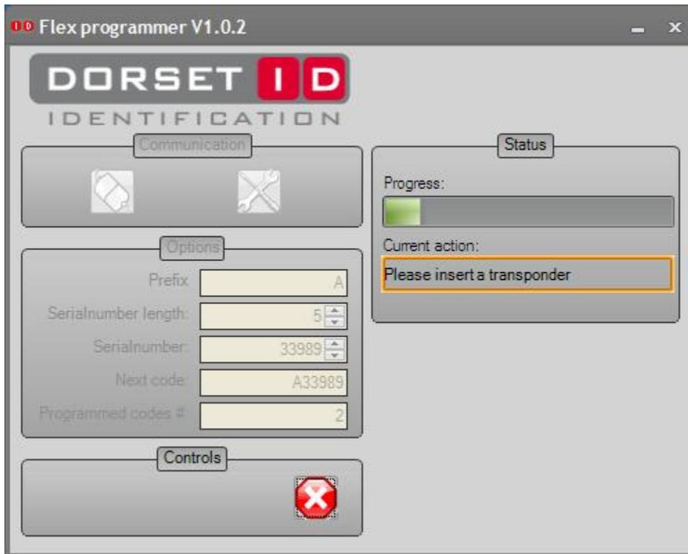
The number will increment by 1 every time you insert a transponder into the Programmer.
